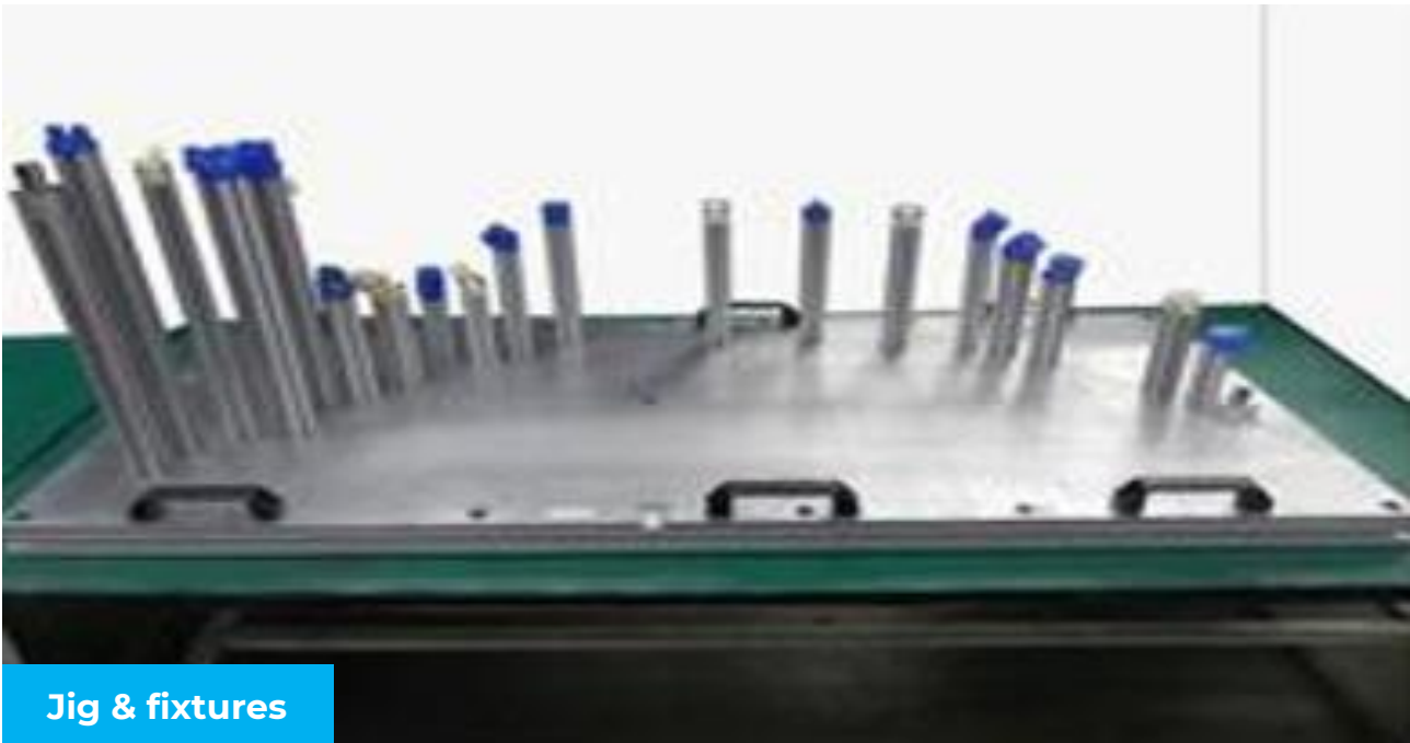
Jig : Wings Inspection Jig
